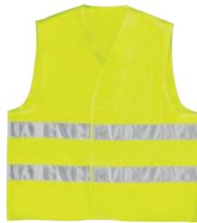
Vest. Fastening with velcro band. High visibility: Class 2. Parallel assembly. Polyester fabric. Retro-reflective sewn bands.
