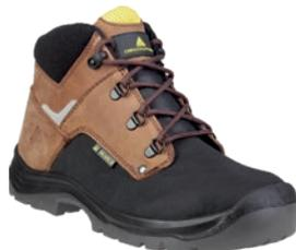
Upper: Cow leather, water resistant treatment S3 and PU-coating suede split leather. Lining: Absorbent 3D mesh. Insole: Removable premolded - Polyester on EVA. Outsole: Injected - Dual-density PU.
