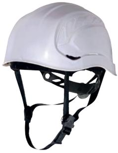
ABS safety helmet. Mountain helmet style; without visor for the best vertical vision. Less encumbrance. Light. Polyamide cradle: 3 textile bands with 8 fixing points. Thermoformed sweat band. Innovative adjustable ROTOR system : head sizes 53 to 63 cm. Sold with 3 point chin strap. Specially designed for working at height. Electrical insulation up to 1 000 V.A.C. or 1 500 V.D.C.
