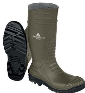
Upper: PVC. Lining: Polyester. Protection of the malleoli. Front and back protection toe bumper. Rear removal lug. Protective toe cap: stainless steel. Anti-perforation mid sole: stainless steel. Sole: PVC - Nitrile.
